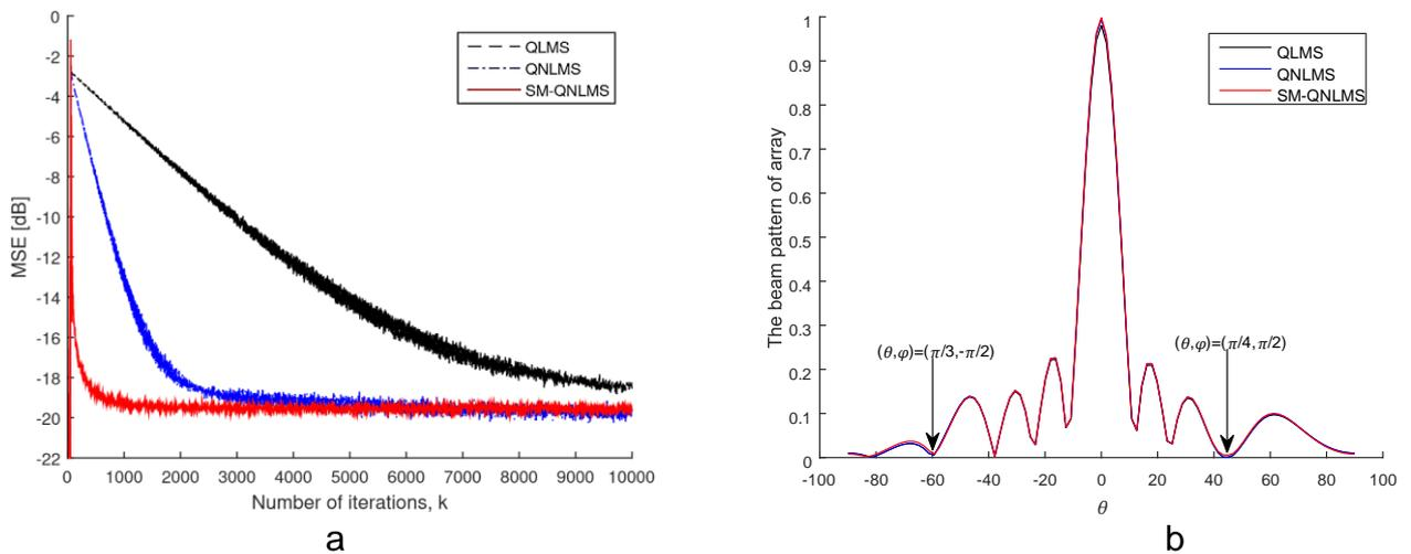
Fig. 2 (a) The MSE learning curves of the QLMS, the QNLMS, and the SM-QNLMS algorithms; (b) Beam patterns of the QLMS, the QNLMS, and the SM-QNLMS algorithms when DOA of the desired signal is  $(\theta, \phi) = (0, \frac{\pi}{2})$
