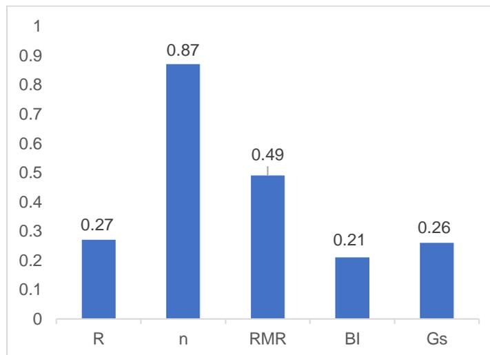
Fig. 25. Strength of input Parameters in UCS Prediction
