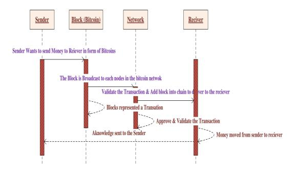
Fig. 1. Sequence Diagram for Working Mechanism of Blockchain
